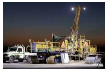
Diamond drilling on Lake Lefroy
