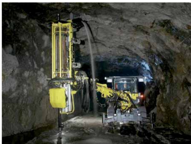
Simba drill rig – drilling bench holes 95 3West
