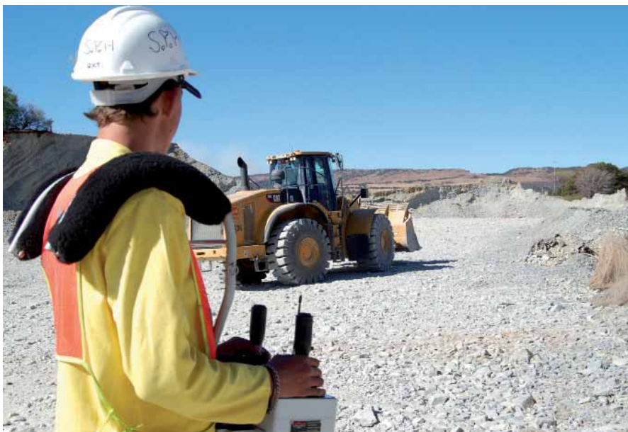
Remote loader used by SPH at Driefontein in the mining of a surface rock dump in an area where sinkholes occur
