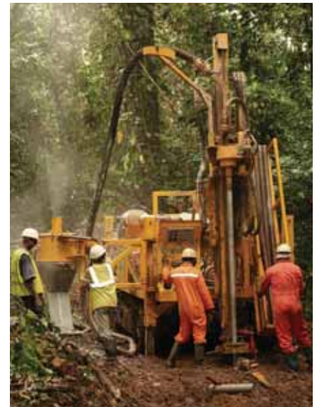
Air-core exploration drilling at Nohokoa
